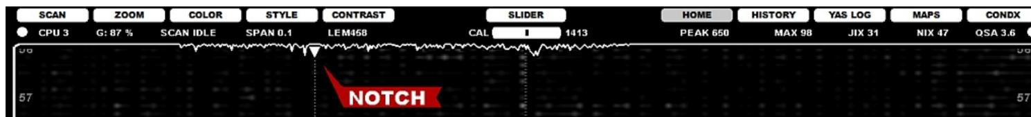
You cannot directly re-adjust the position of AUTONOTCH, but those notches can be tuned in AUDIO WINDOW. Notching (auto & manual) always removes a part of the "raw audio" so it is a challenging game. Some experienced DXers are very critical about classic autonotching but they can accept this type of "safe autonotching", and can keep AUTONOTCH always on by default.
