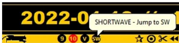
By default, the new SW frequency is 12095 kHz (used by BBC) but JAGUAR remembers the last tuned SW frequency, and when this SW button is clicked next time, the last tuned SW frequency will be used, instead of 12095 kHz.
