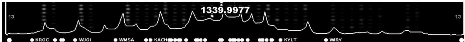
In addition to the FLAGS, public offsets are also displayed as "offset balls" below the SPECTOR curve. These dots are always visible but due to large numbers of offsets many of them are overlapping and all the names can't be shown. By default the positions are based on the MWLI offsets, but if you have FLAGS open, also the Kapsi offsets are included. Clicking any of the balls tunes the playback to that exact offset and right clicking the ball triggers the STATION MENU.
