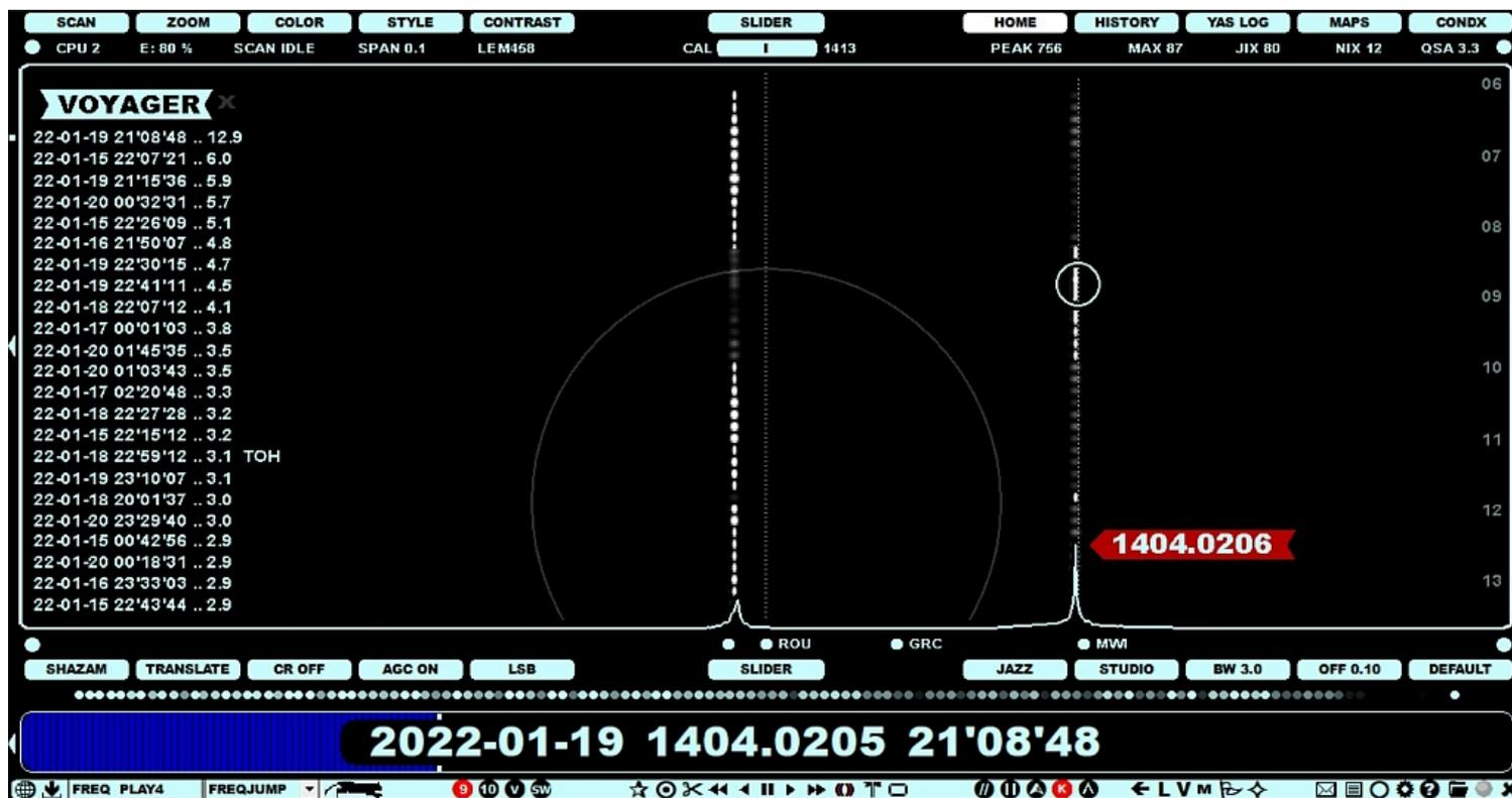
And indeed: for a short period MBC Chitipa playing Congolese rumba ("Point Faible" by Commandant Josky as identified by Shazam) is the only station audible on 1404 kHz. If HOMESCAN is active, it draws the spectrum visible on the display immediately after jumping to that file (no need to listen the file) and also it confirms that Malawi is the strongest station on this frequency for almost two minutes (CATWALK's white track is always attached to the strongest carrier of the frequency).
