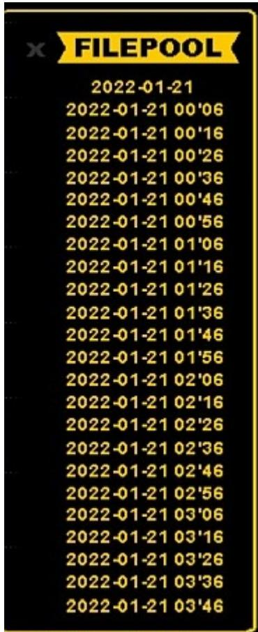
The FILEPOOL can be shown on every graphics display as a text overlay on the right edge of the display. The contents can be scrolled up/down, you can quickly open any file from it, and you can also change days quickly.
