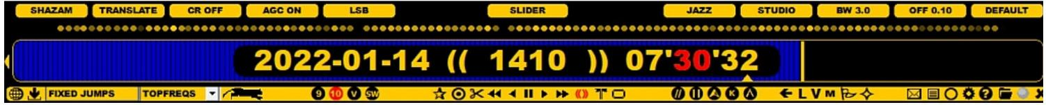
Pressing the TAB key will rotate the active scrollable objects: MONTH > DAY > FREQUENCY > HOUR > MINUTE > SECOND.
