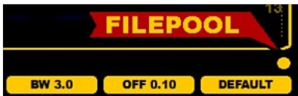
You can open/close the FILEPOOL by pressing ALT-O or by clicking the FILEPOOL button on the lower right corner of the graphics area.
